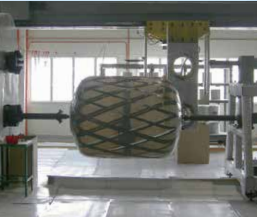
Digital Controlled Filament Winding
